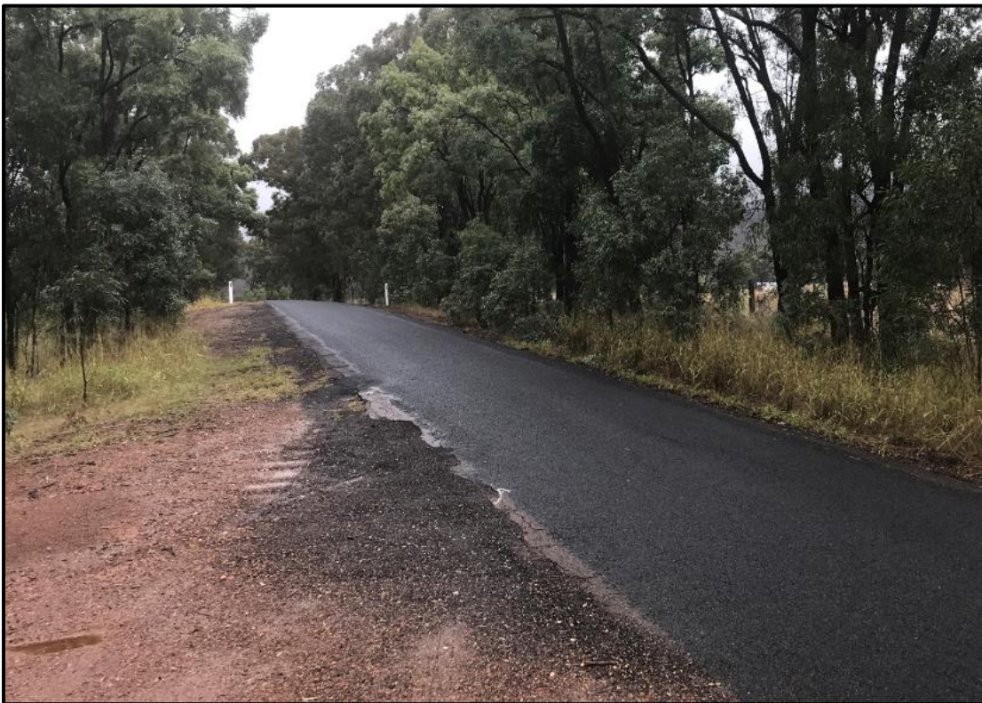
Photo 4 – Visibility for a car driver to the left is 124 metres. Distance exceeds 200 metres for truck driver line of sight when exiting the subject site
